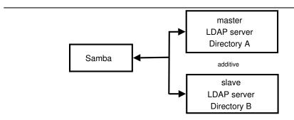
**Figure 6.5.** Samba Configuration to Use Two LDAP Databases - The result is additive.
