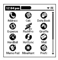
When power is restored, the FlashPro backup icon will appear. Launch FlashPro to restore FlashPro to RAM. The RAM copy will run automatically.
