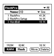
Launch FlashPro. A list of the current files in RAM will be displayed. Select a file to move to flash memory. Tap the "Move" button.
