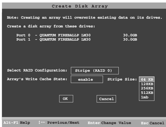
Figure 13. Create Disk Array Display, RAID 0 Example
