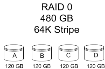
Figure 1. RAID 0 Configuration Example
