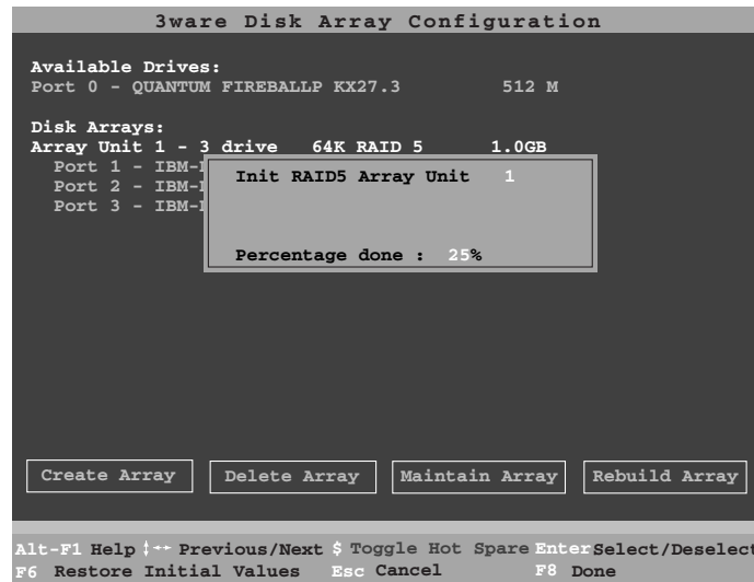
Figure 15. BIOS Initialization Screen for RAID 5
