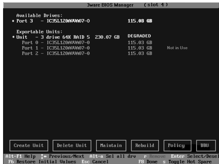
Figure 49. Select Available Drive to Replace Faulted Drive
