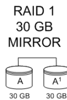
Figure 2. RAID 1 Configuration Example
